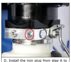
D. Install the iron plug from step A to the oil outlet port on the left side.
