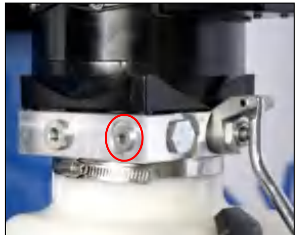
D. Install the iron plug from step A to the oil outlet port on the left side.
