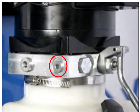
D. Assemble the socket plug by Step A to this left oil outlet port.
