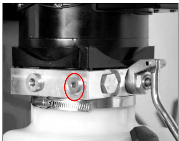
D. Assemble the socket plug from step A to this left oil inlet port.
