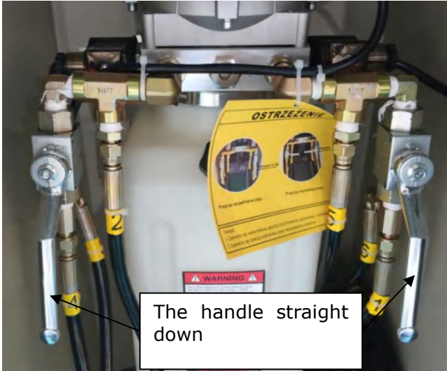
Oil Filling Position Fig. 29
