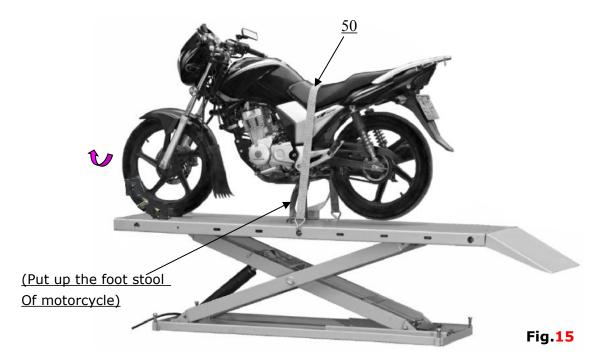
**4. To lower the lift:** Rise the lift few seconds. Rotate the safety lock handle downward (see Fig.16) to release the safety device. After the safety device is released (see Fig.17), press **DOWN** button to lower the lift.
