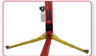
4 three-stage telescoping arms accommodate more vehicles
