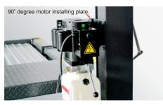
90° degree motor installing plate
