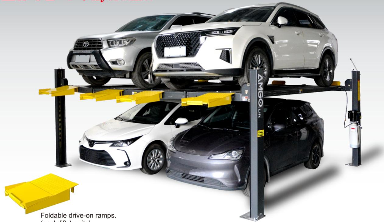
Foldable drive-on ramps. (each lift 4 units).
