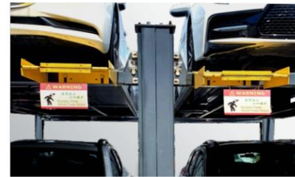
Special structure design to allow back-to-back installation.
